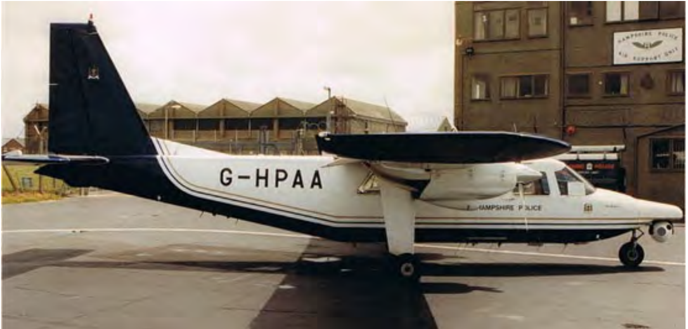
Hampshire Police BN2B-20 Islander - G-HPAA, with a nose mounted Leo 400 EO /IR camera turret.
